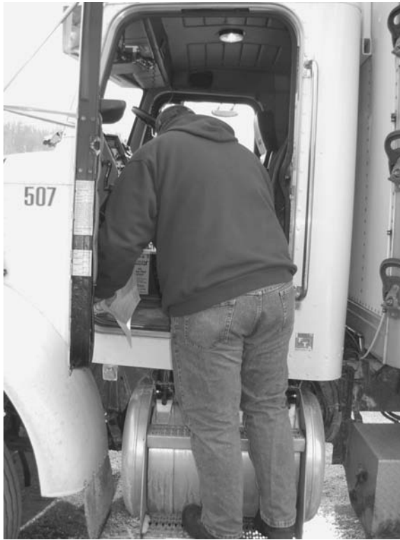
FIGURE 16.2 Drivers can slip and fall while mounting and dismounting vehicles.
