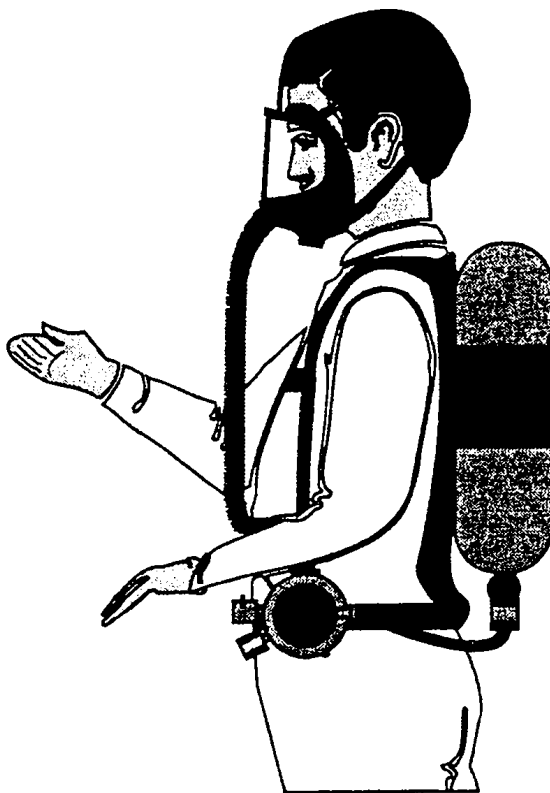
FIGURE 24.12 Example of a self-contained breathing apparatus (SCBA). (Courtesy of the National Institute for Occupational Safety and Health.)
