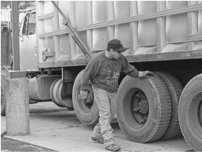
FIGURE 16.4 Another layer of safety is pre-operational inspection by drivers.
