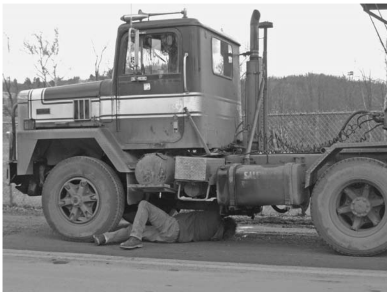
FIGURE 17.1 Operators need to conduct pre-shift inspections and constantly look for potential problems such as this broken exhaust.
